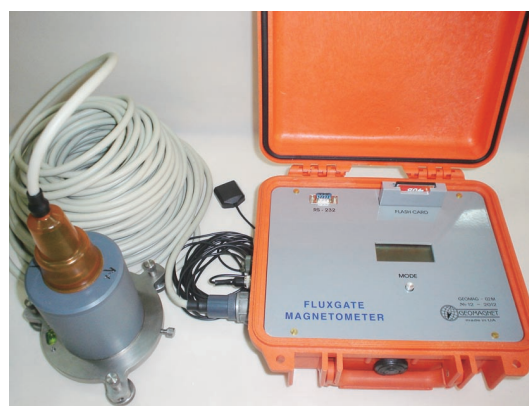
Figure 3 A regular fluxgate magnetometer running at Zhongshan Station, which consists of an electronic unit, a sensor and a GPS antenna. A signal cable connects the sensor and the electronic unit. Additionally, a personal computer is used to monitor observation and register data, which is connected to the electronic unit via a RS-232 serial port.
