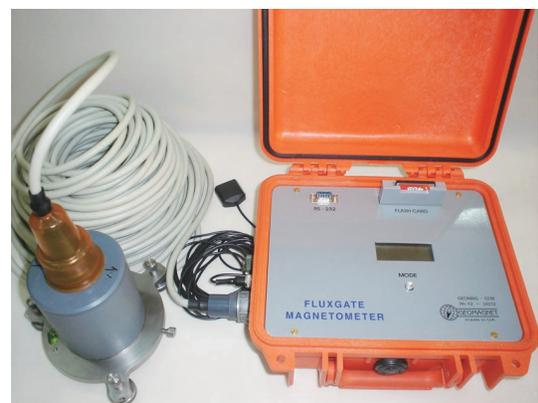
**Figure 3** A regular fluxgate magnetometer running at Zhongshan Station, which consists of an electronic unit, a sensor and a GPS antenna. A signal cable connects the sensor and the electronic unit. Additionally, a personal computer is used to monitor observation and register data, which is connected to the electronic unit via a RS-232 serial port.
