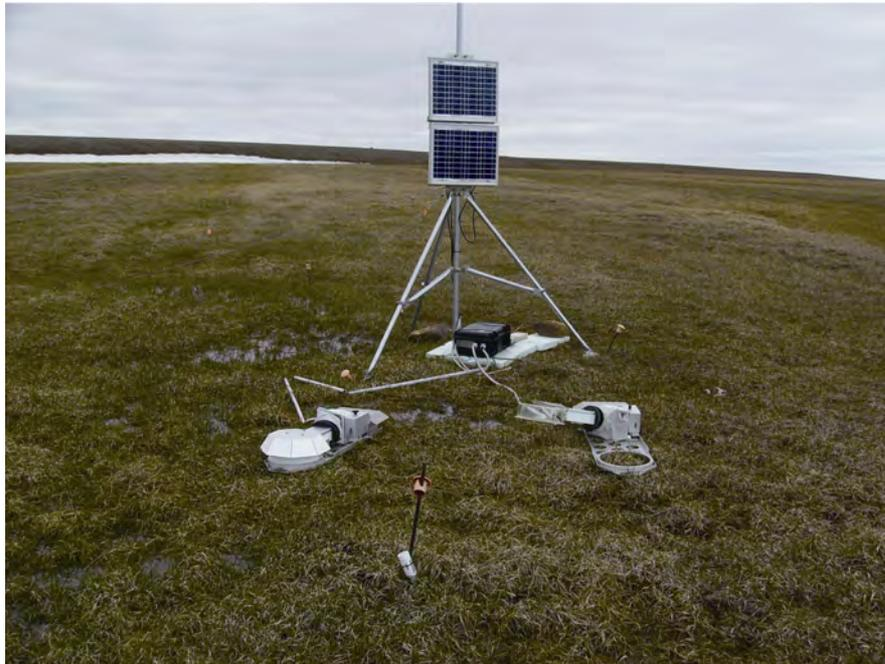
**Figure 2** Pair of ADC ACE autochambers installed in the Muskox catchment site at the Cape Bounty Arctic Watershed Observatory taken by Dr. Neal Scott in 2017; transparent (right) and opaque (left).
